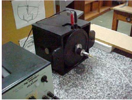
Figure 2: The accelerometer mounted on the electrodynamic shaker
