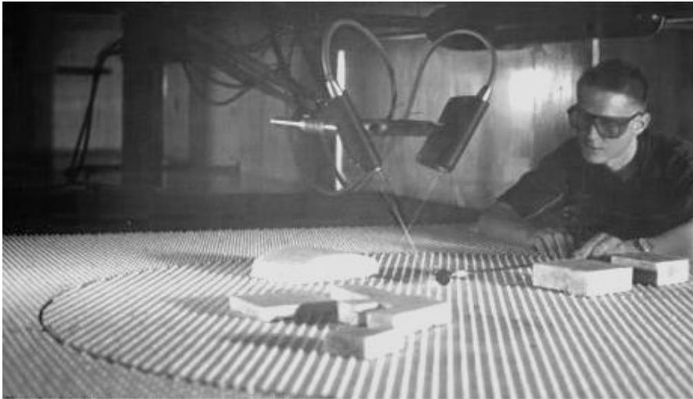
Figure 1. Officer Cadet David Nelson using laser Doppler velocimetry to measure runway turbulence generated by a model of nearby hangar and business park at Canberra Airport.
